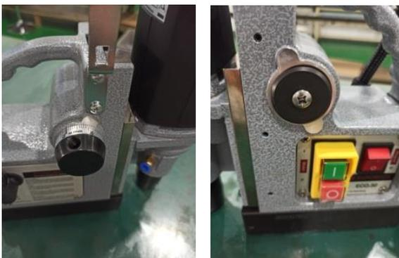
4. Remove the oil tank bracket before fitting the handles.
