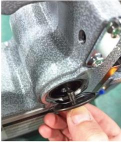
2. Take out the shaft and washer on the standard operating side. Don't forget any rings or bearings (ECO.40S(+)) and F16(+)) on the non-operating side.
