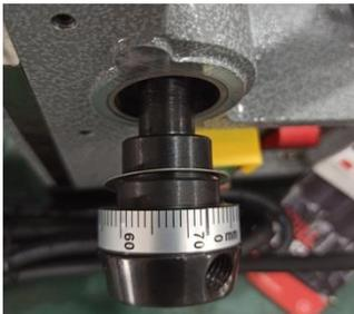
3. Reinstall the parts on reverse sides and fasten the shaft with the same screw and screwdriver.
